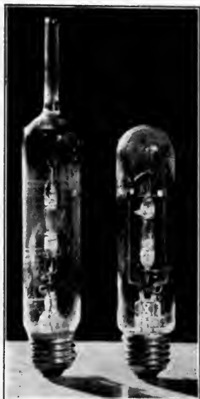
FIG. 2. (a) H3X arc modified for forced-air cooling; (b) Normal H3X arc.
